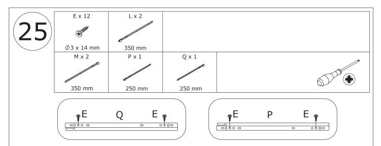
Fix runner(P) and (Q) to board 23 and 24 with screw(E) as shown. Fix runner(L) and (M) to board 19 and 20 with screw(E) as shown.
