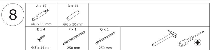
Screw eccentric rod(A) and insert wooden dowel(D) into board 7 and 8 as shown. Fix rail(P) and (Q) to board 7 and 8 respectively with screw(E) at first. Screw eccentric rod(A) into board 11 as shown.
