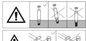
Screw eccentric rod(A) and insert wooden dowel(D) into board 12 and 13 as shown.
