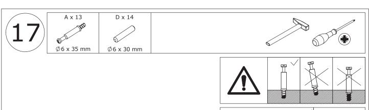
Screw eccentric rod(A) and insert wooden dowel(D) into board 1 and 2 as shown. Connect board 1 and 2 as shown.
