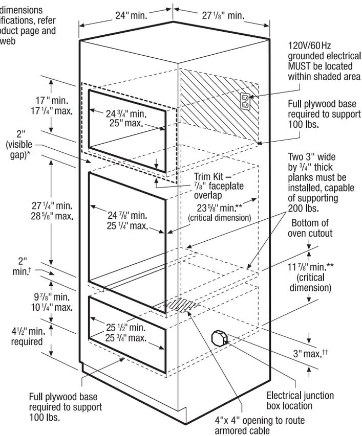
\* Minimum 2 7/8" clearance required from bottom of Built-In Microwave cutout to top edge of Wall Oven's faceplate, leaving a 2" visible gap between both product faceplates.
