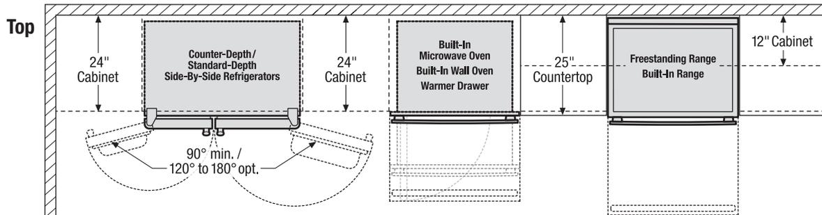
When installing side-by-side refrigerator adjacent to wall, cabinet or another appliance that extends beyond front edge of unit, 20" minimum clearance recommended to allow for optimum 120° to 180° door swing, providing complete drawer/crisper access and removal.
