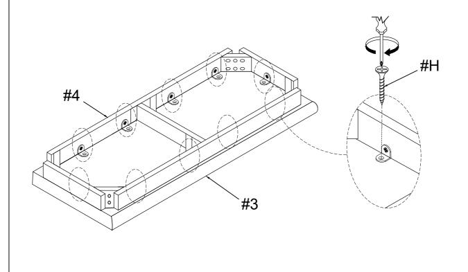
Do not tighten screws until completely asembled.
