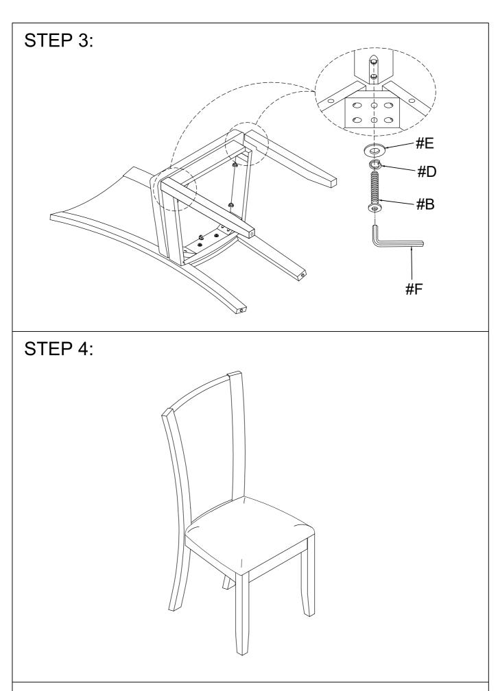
Tighten all screws until completely asembled.
