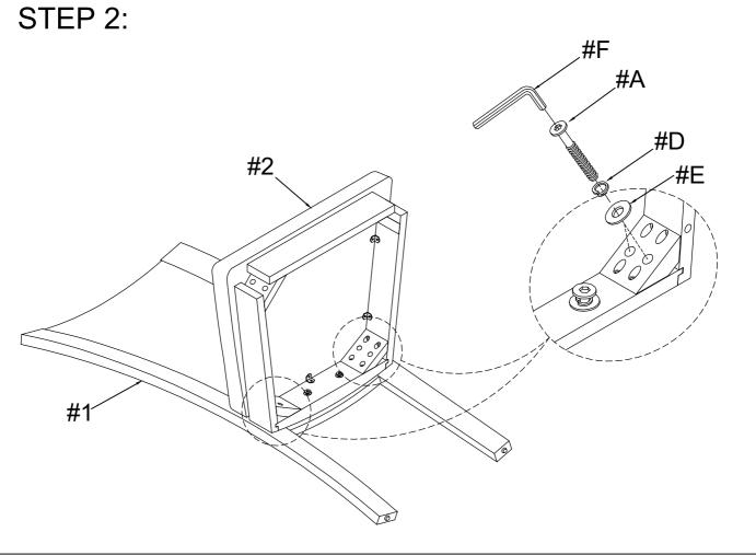
Do not tighten screws until completely asembled.
