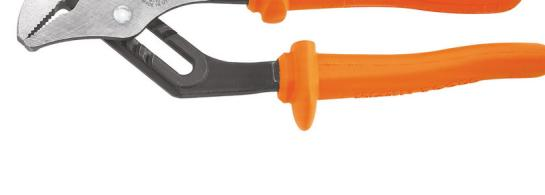
These Klein Tools 10-Inch Insulated Pump pliers feature integral guards to help prevent accidental contact with conductive wire and a wide jaw capacity for versatility. They are individually tested to exceed the IEC 60900 and ASTM F1505 standards, for insulated tools and clearly marked with the official 1000-Volt rating symbol. The handles feature two layers of insulation to provide protection against electric shock.
