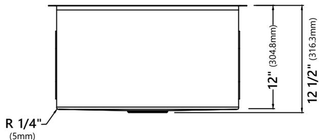
**NOTE:** It is not recommended to install this sink with a negative reveal. Doing so will prohibit the use of any workstation accessories as they will not fit.
