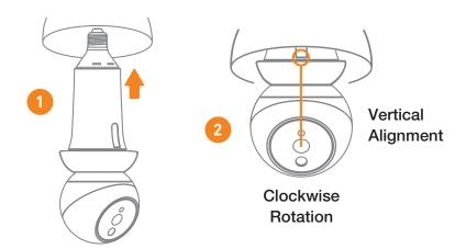
Screw in the device by placing it into a lightbulb socket, then, gently turn clockwise until it is secure.
