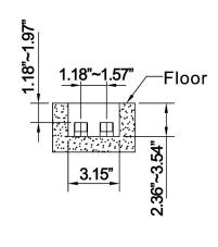
4.Connect the inlet tube like the drawing.
