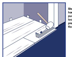
Step 2: Use hammer and pull bar to lock this piece of flooring
