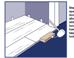
Step 1: Undercut space under door jamb to allow flooring to slide freely. Tap long edge with hammer and tapping block to lock long edge.
