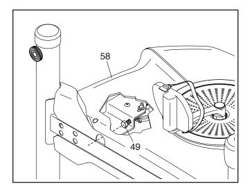
Using an M10 socket wrench with an extension (not included), reach into the opening in the bottom of the Right Shield (58) and tighten the M10 x 50mm Screw (49) a few turns until the Drive Belt (not shown) is tight; **do not overtighten the Drive Belt.**
