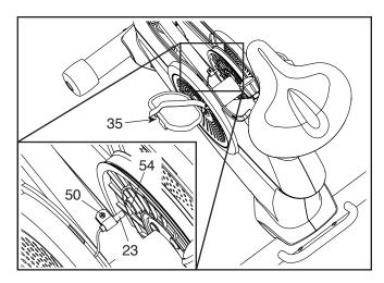
Next, rotate the Left Crank Arm (35) until a Magnet (54) is aligned with the Reed Switch (23). Slide the Reed Switch slightly toward or away from the Magnet. Then, retighten the M4 x 19mm Screw (50).
