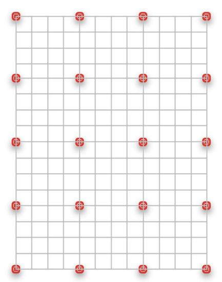
For our 2" Steel Mesh Chair, we recommend placing a chair every 24" in each direction. Simply pull the mesh up off the ground and snap the chair's clips onto the mesh's wire crossing from the bottom.
