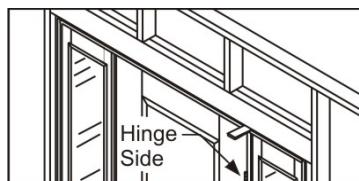
Shim directly over hinge side mull post. Using a 6 foot level, recheck hinge mull post to ensure it is plumb and straight. Finish driving screw tight.
