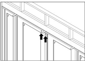
When installing a French door with active sidelites, place temporary shims above the center of the head frame, between the strike plate screws.
