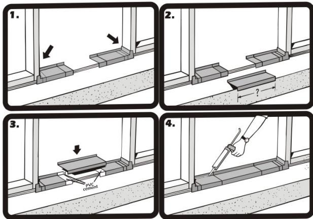
**Note:** Use only the PVC cement provided in the sill pan kit to glue the pieces together. The sill pan must be sealed to the sub-floor using a high-quality hybrid polymer, elastomeric or polyurethane sealant; Therma-Tru recommends OSI QUAD MAX, but do not apply sealant to the bottom of the sill when using a sill pan.
