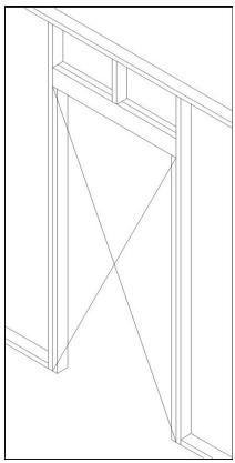
Check to be sure the framing walls around the opening are in the same plane. Do this by performing a "string test" for plumb.
