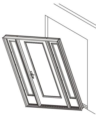
Lift the unit up. With top edge tilted away from opening, center the unit and place sill down onto sill pan or caulk beads and tilt into opening.
