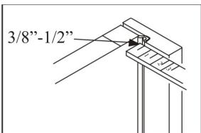
Adjust lock side mull post so that the weatherstrip contacts the door surface equally at the top, middle, and bottom, an even 3/8" – 1/2" when fully closed. Pre-drill and insert a screw through the frame into the header, on each side of the lock mull post
