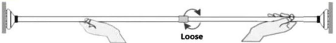
**3.** Make sure the pole is parallel; press down to see if it's loose. Confirm ok, and the installation is complete.
