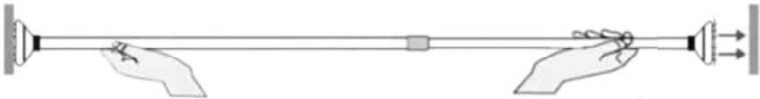
**2.** Hold the left tube and do not move; tighten the right tube clockwise.
