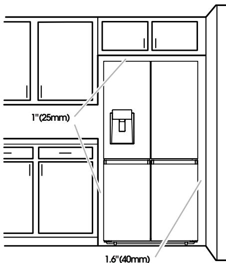
To ensure proper ventilation for your refrigerator, allow for a 1"(25mm) space on each side and at the top. Allow at least 2.0"(51mm) between back of cabinet and the wall. If your refrigerator has an ice maker, allow extra space at the back for the water line connections.
