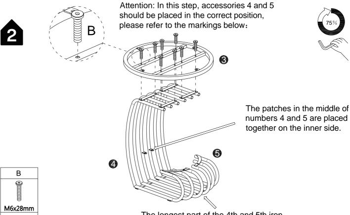
The longest part of the 4th and 5th iron pipes are pressed together on the inside.
