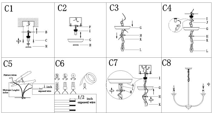
Step C1: .Attach single bar (B) to outlet box with mounting screw (C). The side of single bar marked "GND" must face out. Then unscrew collar ring (H) from collar loop (I)
