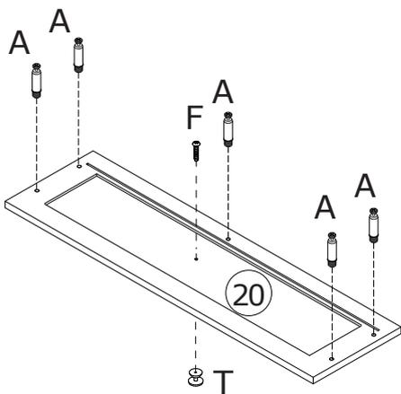
Fix knob(T) to No.20 and No.29 plate with screw(F).
