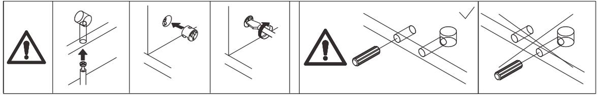
Connect the two components with wooden dowel(D) and turn cam lock(B) clockwise to tighten as shown.
