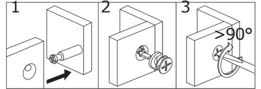
Attach No.28, No.27 and No.25 plate to No.17,19 plates respectively, turn cam lock(B) clockwise to tighten as shown.
