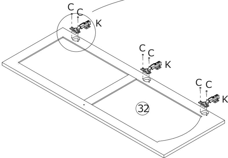
Fix hinge(K) to No.30,31,32 plate with screw(C) as shown. Please don't use an electric screwdriver or use force to rotate, may cause crack.
