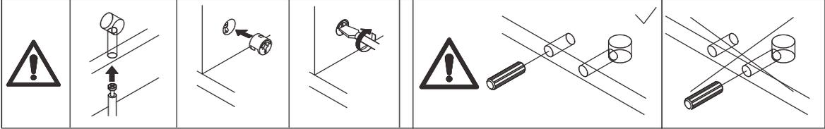
Attach No.1 plate to No.2,3,4 plates with wooden dowel(D) and turn cam lock(B) clockwise to tighten as shown.
