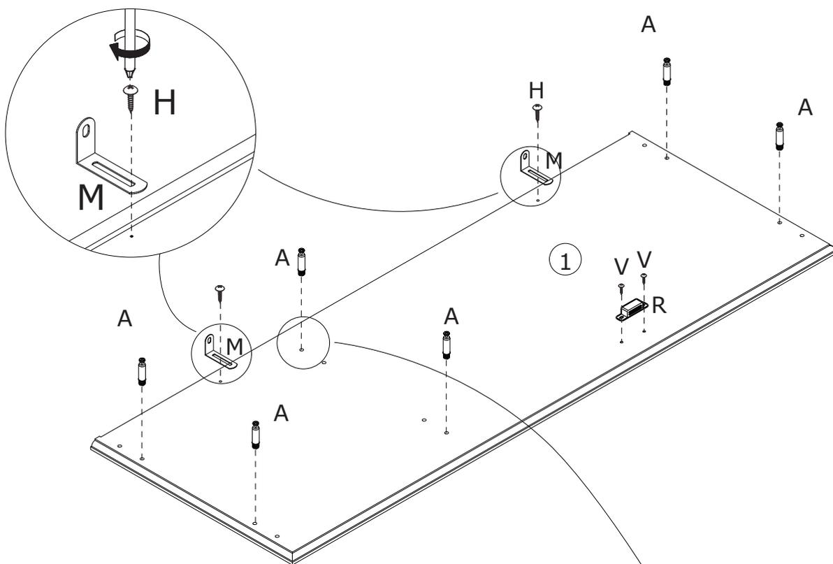
Insert quickfit screw(A) into corresponding holes in No.1 plate with a screwdriver as shown.
