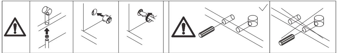
Attach No.9 plate to No.13 with wooden dowel(D) and turn cam lock(B) clockwise to tighten as shown.
