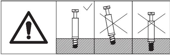
Attach No.17,19,22 plates to No.18 with screw(G) as shown.
