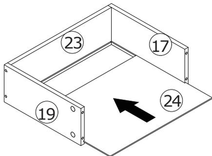
Slide No.24 and No.36 plates into available slots respectively as shown.
