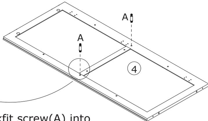
Insert quickfit screw(A) into No.3 and No.4 with a screwdriver as shown.
