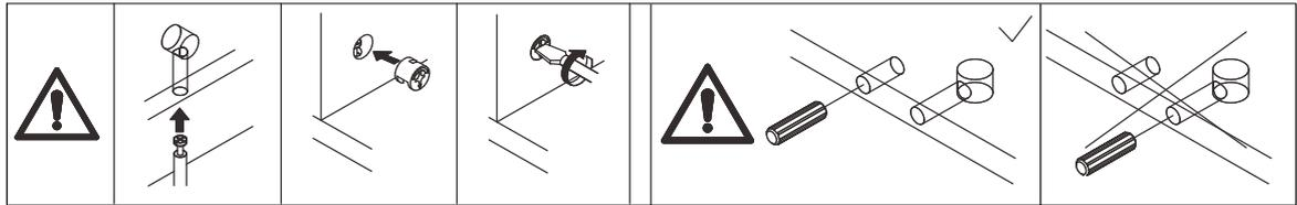
Connect No.3 and No.4 plate with No.5 using wooden dowel(D) and turn cam lock(B) clockwise to tighten as shown.
