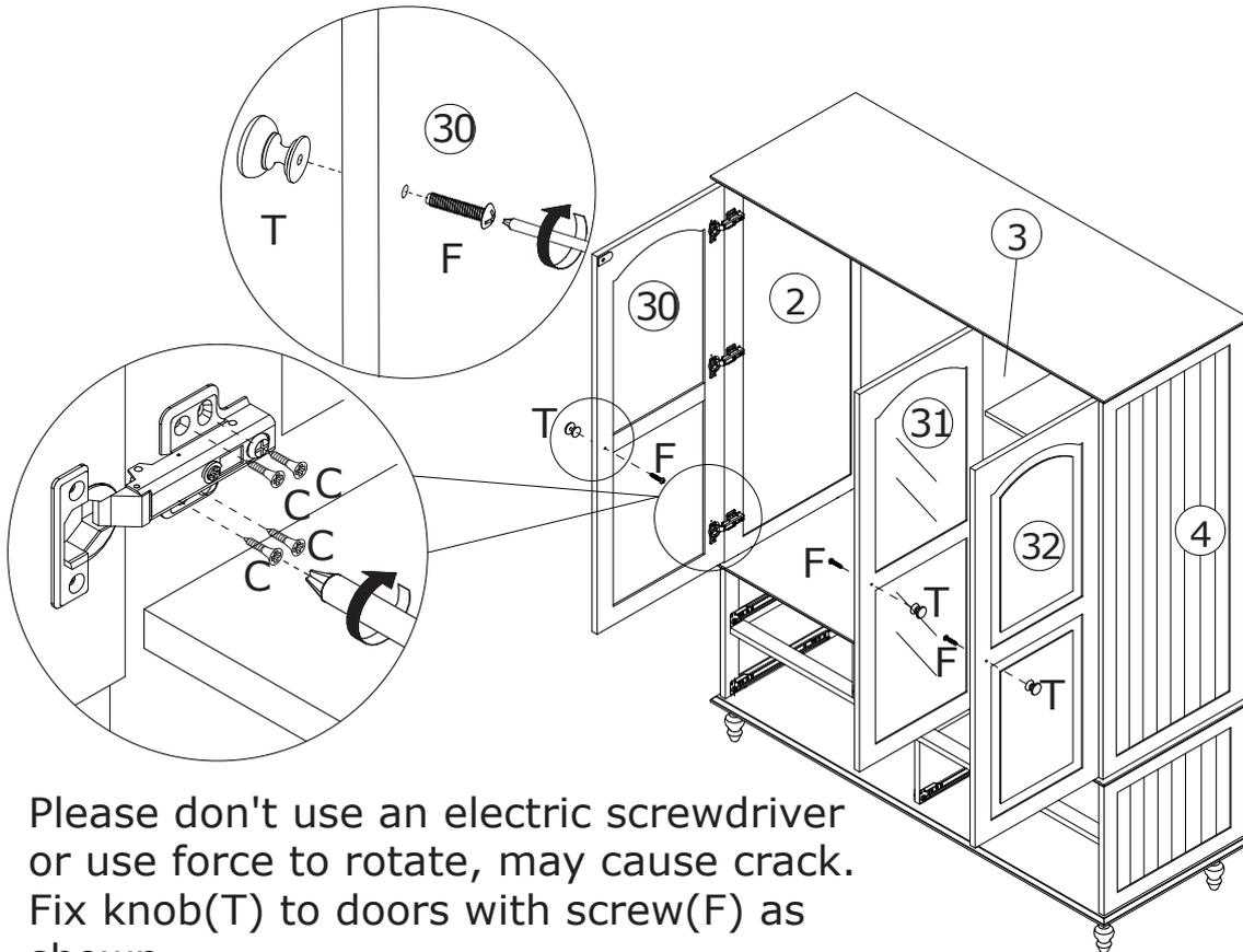
Attach No.30 to No.2, No.31 to No.3, No.32 to No.4 plate by fixing hinge with screw(C) as shown.
