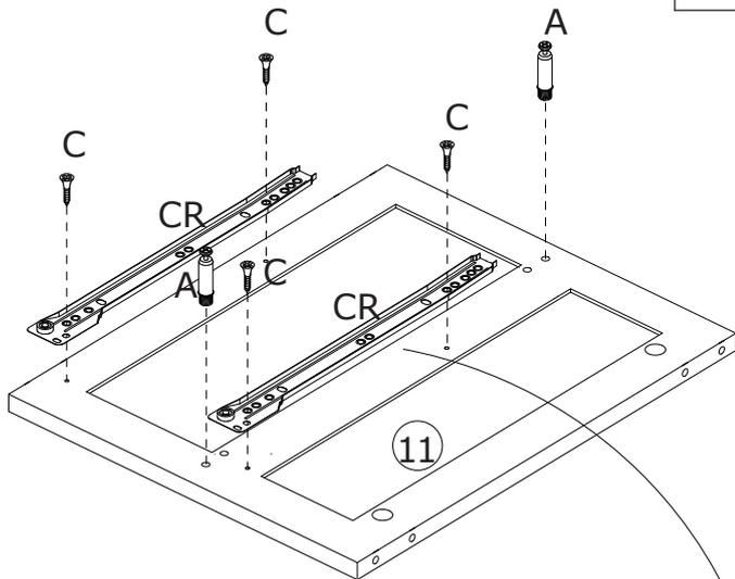
Fix slide rail(CR) to No.11 plate with screw(C), fix slide rail(CL) to No.10 plate with screw(C) as shown.
