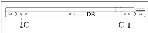
Fix runner(DL) and (DR) to No.19 and No.17 plates respectively with screw(C) as shown.
