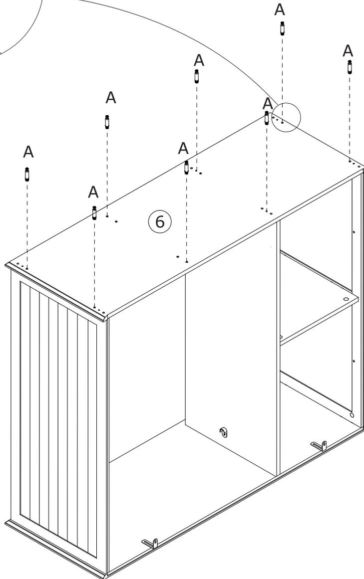
Insert quickfit screw(A) into corresponding holes in No.6 plate with a screwdriver as shown.
