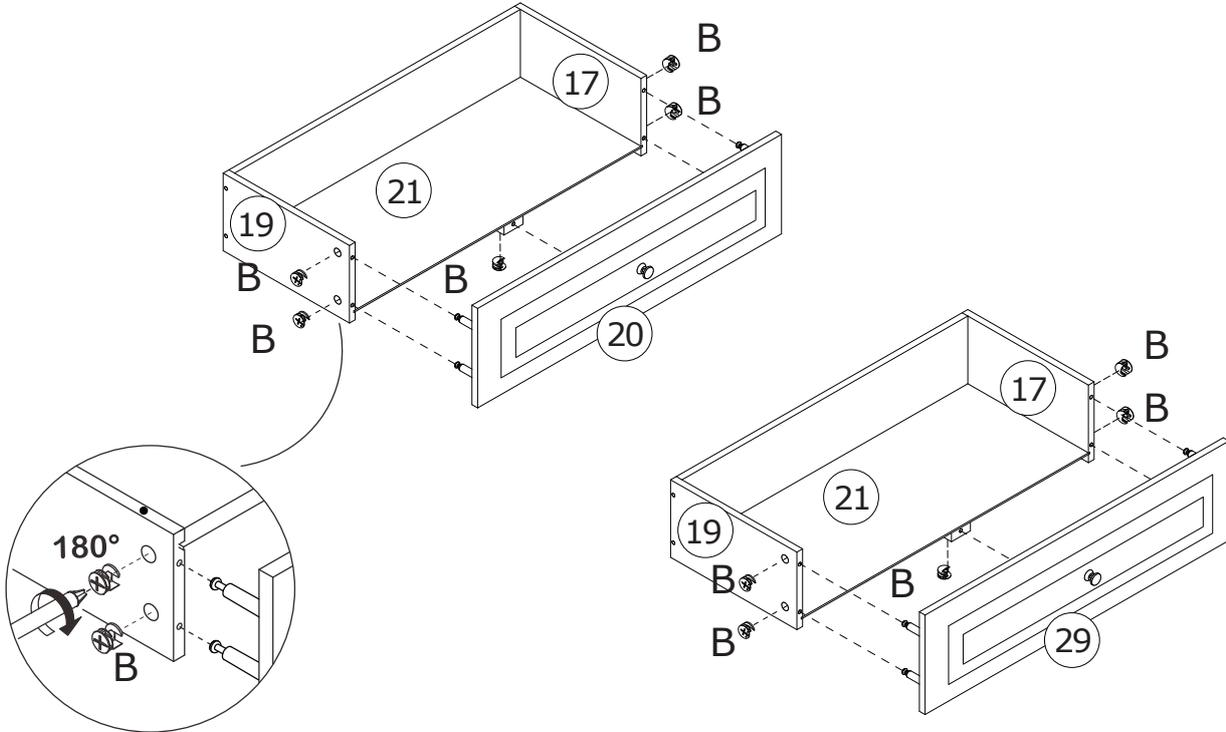
Attach No.20 and No.29 plate to No.17,19 plates respectively, turn cam lock(B) clockwise to tighten as shown.
