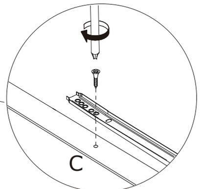
Insert quickfit screw(A) into No.10 and No.11 plates with a screwdriver as shown.
