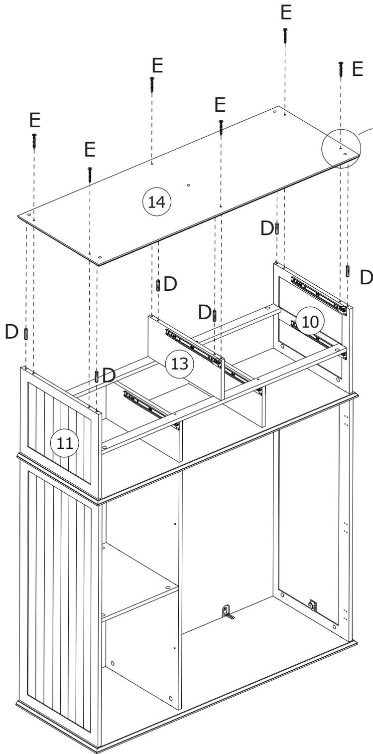
Cover No.14 plate to No.11,13,10 plates with wooden dowel(D) and then fix with screw(E) as shown.
