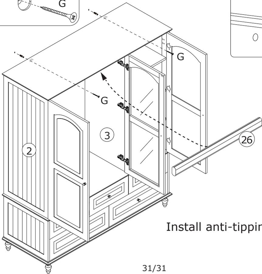
Install anti-tipping device as shown.
