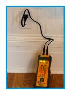
Hold the Receiver near the Transmitter to verify connection, confirmed by the lightning bolt symbol.
