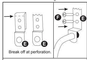
Use a drill (not included) to pre-drill holes if you are installing this shoe rack onto drywall or soft wall. Insert wall anchors (H). Use a Phillips screwdriver (not included) to tighten screws (F) into wall.
