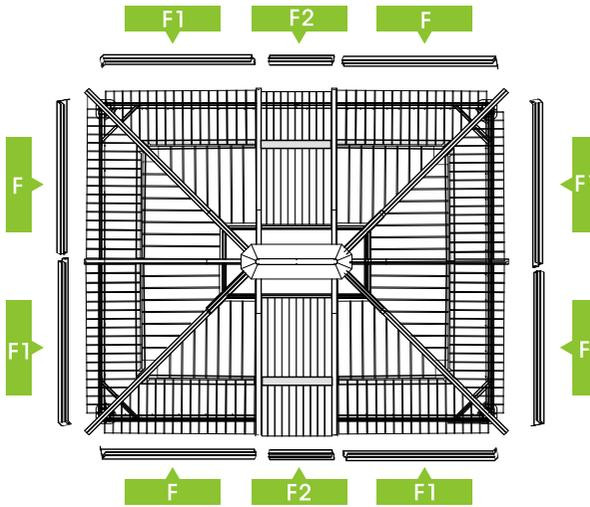
**26** Use 6 parts "X" and 6 screws "U" to fix parts "F" and "F2". Use 4 parts "Y" and 4 screws "U" to fix parts "F" and "F1".
