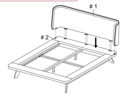
Use bolt assembly of bolt (#A) with spring washer (#F) and flat washer (#E) to attach the center of headboard (#1). Then secure the wings.
