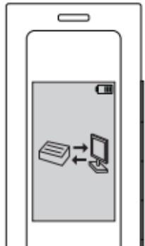
**Note:** Please do not disconnect the X200 by removing the Micro-USB data cable. This can damage the files stored in the Recorder's internal memory.
