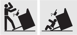
**⚠ WARNING:** If your range is removed for cleaning, servicing or any reason, be sure the anti-tip device is re-engaged properly when the range
