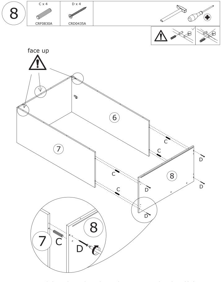
Attach board 8 to board 6 and 7 using wooden dowel(C), and fix with screw(D) as shown.
