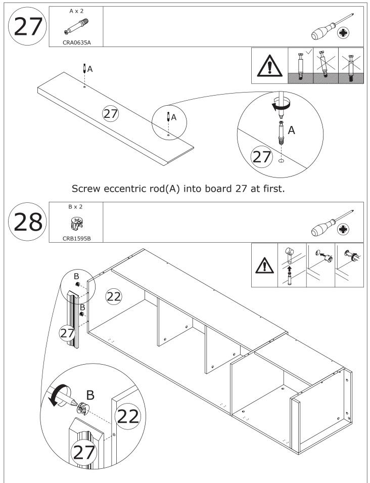
Attach board 27 to board 22, add cam lock(B) into board 22 and turn clockwise to tighten as shown.
