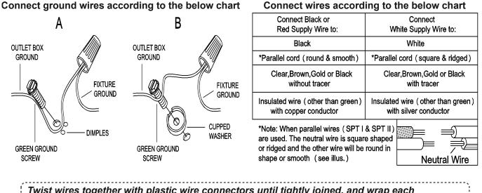
Twist wires together with plastic wire connectors until tightly joined, and wrap each connector with approved electrical tape. Be sure that no wire strands are exposed and then carefully tuck all wires into the outlet box.
