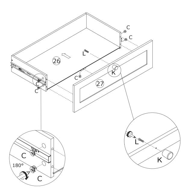
Attach board 27 to the component, turn cam lock(C) clockwise to tighten as shown.
