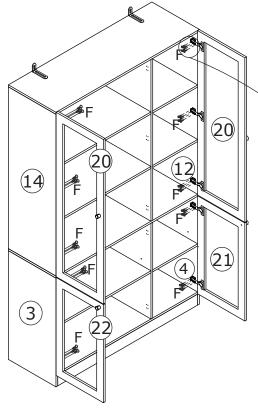
Assemble door 20 to unpper cabinet by fixing hinge with screw(F) as shown.
