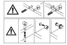
Attach board 5 to board 1 and 2, add cam lock(C) into board 1,2 and turn clockwise to tighten as shown.
