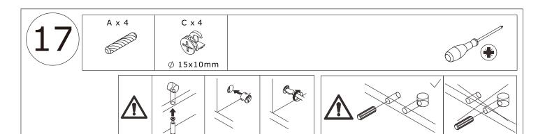
Insert wooden dowel(A) into board 23, 26 and 28 at first.
