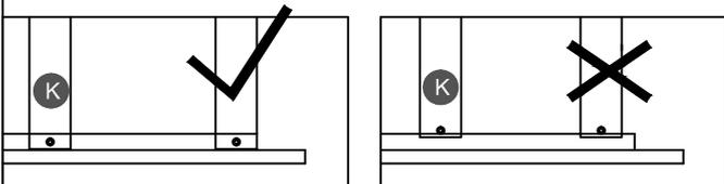
Note: Do not lock the screws of the bed slats to the outermost edge of the bed slats, you need to leave a certain space at the edges, otherwise it will cause the board to break
