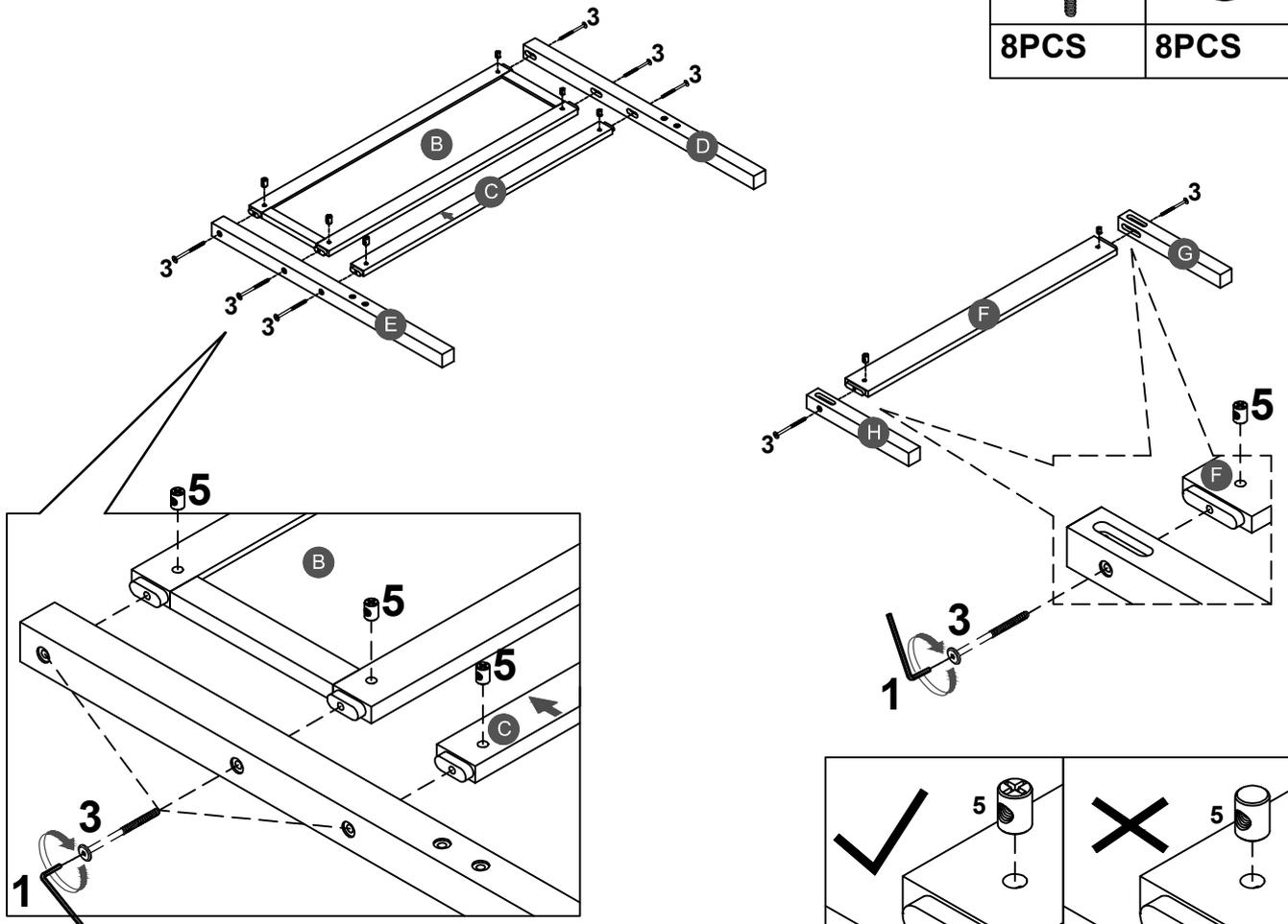
Note: Part 5 will face up with the "x" mark on it, otherwise it cannot be tightened
