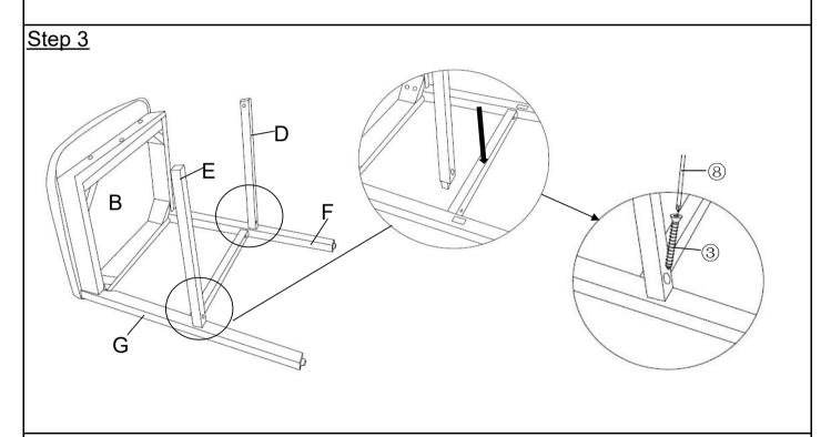
Attach the Left Pedal (D) to the Left Front Leg (F), using Bolt(③) with Screwdriver (⑧). Repeat the step to assemble the Right Pedal (E) to the Right Front Leg (G).
