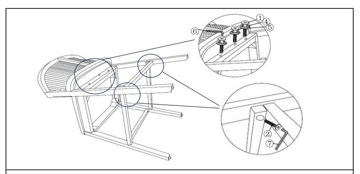
Attach Backrest with Back Leg (A) to assembled frame of Step3 as shown above.
