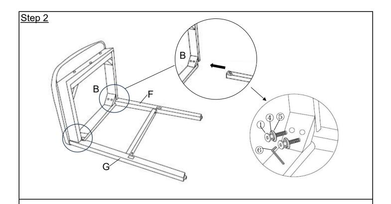
Attach the Leg frame of Step 1 to the Seat (A), using Bolt (①), Spring Washer (④) and Flat Washer (⑤) with Allen Wrench (⑥).
