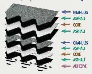
Diamond Cut™ Granules... Add dimension and depth to the shingle with their multifaceted design and light-reflective construction
