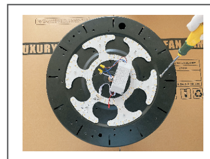
Step 4. Remove the main engine chassis screws.
