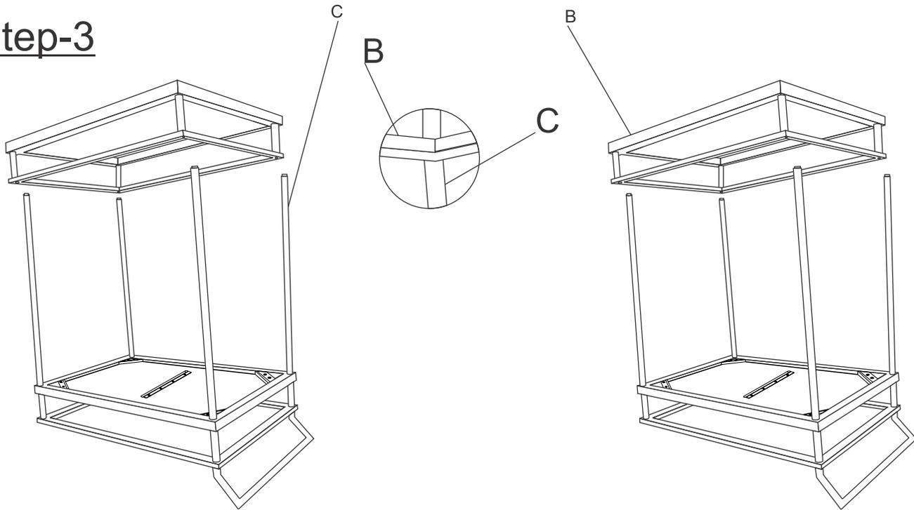
Put the panel (B) in such a way that it will coincide with item (C) at all four corners perfectly.
