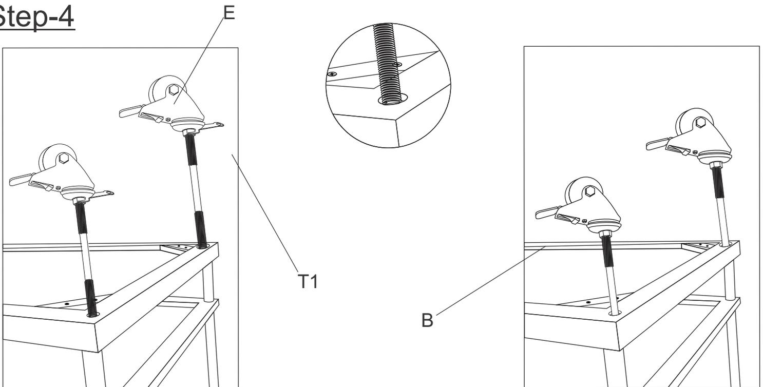
Insert the rod of item (E) into the panel (B) and get it screwed the help of item (T1) all four corners.
