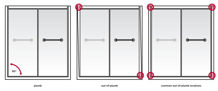
Most Delta Shower Doors are designed to accommodate out-of-plumb conditions up to 3/8". If needed for proper alignment, each roller can be individually adjusted from inside the shower enclosure. Always follow the safety guidelines, and for more detailed instructions, refer to installation guide or contact our Delta Shower Doors Customer Care with questions 800-964-4850.
