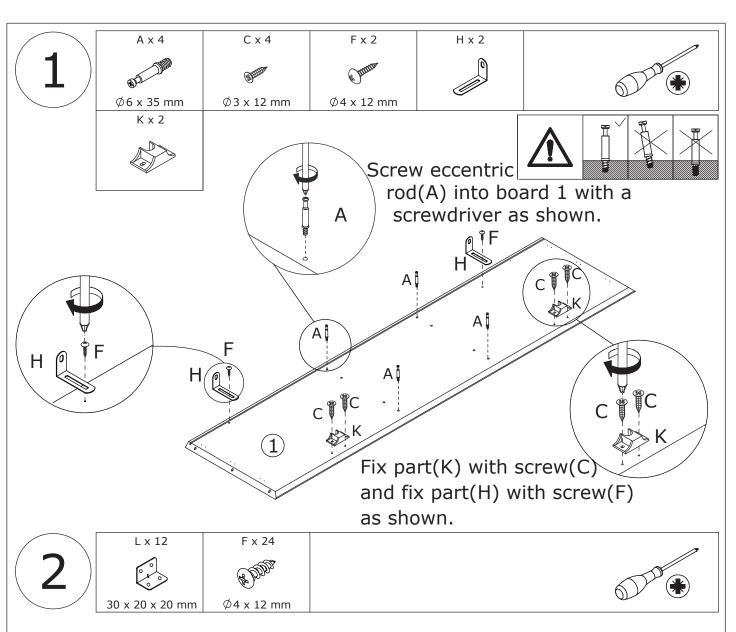
Fix part(L) to board 2 with screw(F) as shown.
