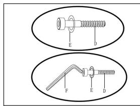
STEP1 PUT THE WASHERS ON THE BOLT IN THE ORDER SHOWN IN THE PICTURE.
