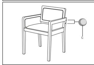
STEP4 PUT THE CHAIR UPRIGHT AND MAKE SURE ALL LEGS ARE LEVEL, THEN FIRMLY TIGHTEN BOLTS WITH ALLEN KEY WHILE THE CHAIR IS UPRIGHT AS PICTURED ABOVE, SEAL THE BOLTS WITH WOODEN DOWELS.
