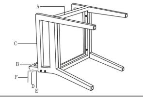
STEP2 ATTACH THE SEAT TO THE RIGHT ARM AND SCREW STEP3 INSERT THE ASSEMBLED SEAT AND ARMS TO THE BACKREST AND SCREW IN THE BOLTS BUT DON'T TIGHTEN COMPLETELY.
