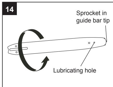
In addition, the guide bar has a sprocket at its tip. The sprocket must be lubricated weekly with a grease syringe to extend the guide bar life. Use a grease syringe to lubricate weekly with chain oil by means of the lubricating hole (Fig. 14). Turn the guide bar and check that the lubrication holes and chain groove are free from impurities.
