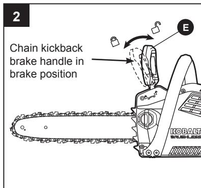
Make sure that the chain brake is working properly before using the chainsaw. The chain kickback brake handle should move back and forth easily.
