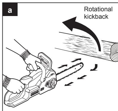
Kickback is the result of tool misuse and/or incorrect operating procedures or conditions and can be avoided by taking proper precautions as given below:
