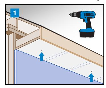
1. From inside the attic locate the area between the soffit joists where you will be installing the soffit vents. Find the center and then drill a hole to mark it.
