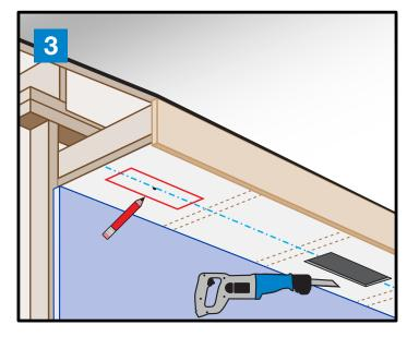
3. On the outside of your home, center the template over each hole that you made in Step 1. Trace around the template. Cut out the template outline with a jigsaw or reciprocating saw.
