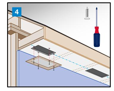
4. Install the vent by centering it over the opening and attaching with four #8 x 1 inch pan-head screws.
