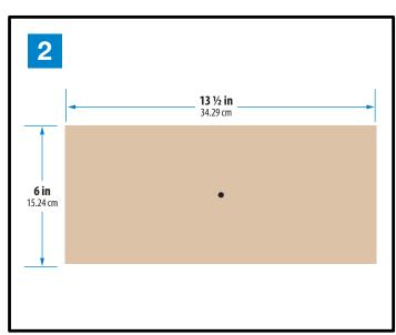
2. Make a 15 in. x 7 in. cardboard template of the **rough opening**. Punch an alignment hole in the center.
