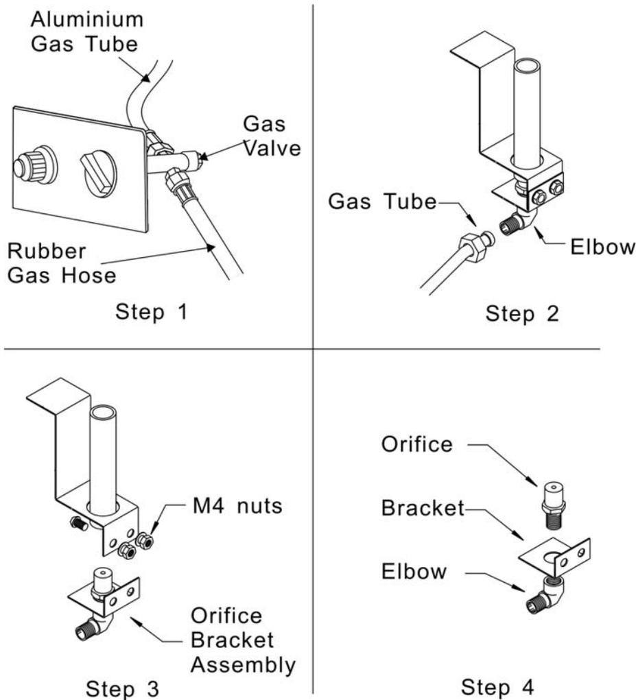
Re-fit the orifice bracket assembly onto the holder using the 2 M4 screws and nuts. Re-connect the aluminum gas tube into the end of the elbow. Connect your Natural Gas supply line onto the gas valve at the control panel. **BEFORE ATTEMPTING TO USE THE FIREPIT, check ALL of the connections for leaks using a solution of soapy water. If a leak is discovered and any bubbles are seen, close the main gas valve and re-tighten ALL the connections. NEVER USE A FLAME TO CHECK FOR GAS LEAKS!**
