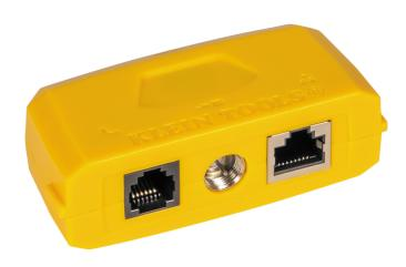
This replacement remote tests, maps and identifies a location in a single step. Use with Klein's Scout® Pro Max Tester (Cat. No. VDV501-770) to test voice, data and video coax cable connections.
