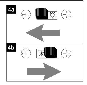
4c. **IMPORTANT:** Reverse switch must be set either *completely* LEFT or *completely* RIGHT for fan to function. If the reverse switch is set in the middle position, fan will not operate.
