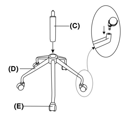
Place the Base (D) on a flat smooth surface. Attach the Castors (E) to the Base (D). Attach Gas Lift (C) to the Base (D)
