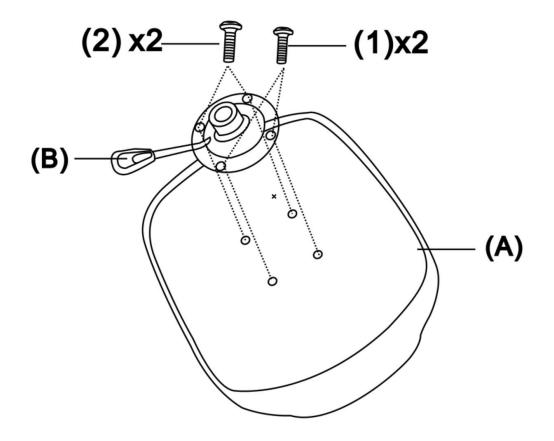
Place the Chair (A) on its back on a flat smooth surface. Attach the Mechanism (B) to the bottom of the Chair (A) with two Short Bolts (1) and two Long Bolts (2). Use Allen Key (3) to tighten.
