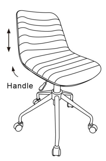
To raise the seat, lift your weight off the seat and reach underneath the right side of the Chair to lift the handle up slowly with a clockwise twisting motion to allow the Chair to rise to desired height. To lower seat, lift the handle slowly with a clockwise twisting motion while seated.
