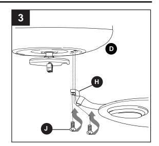
Remove three screws from switch housing plate preassembled on the underside of motor housing (D). Connect male plug from motor housing (D) to female plug from switch housing (F). Make sure plugs connect tightly.
