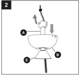
Slip downrod (A) into yoke, align holes and re-install pin (M) and clip (N). Tighten set screws and then tighten nuts on the set screws. Slide yoke cover (E) down until it rests on top of motor housing (D).
