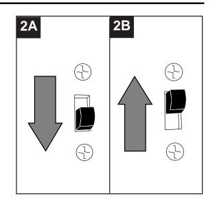
2C. **IMPORTANT**: Reverse switch must be set either *completely UP* or *completely DOWN* for fan to function. If the reverse switch is set in the *middle* position, fan will not operate.
