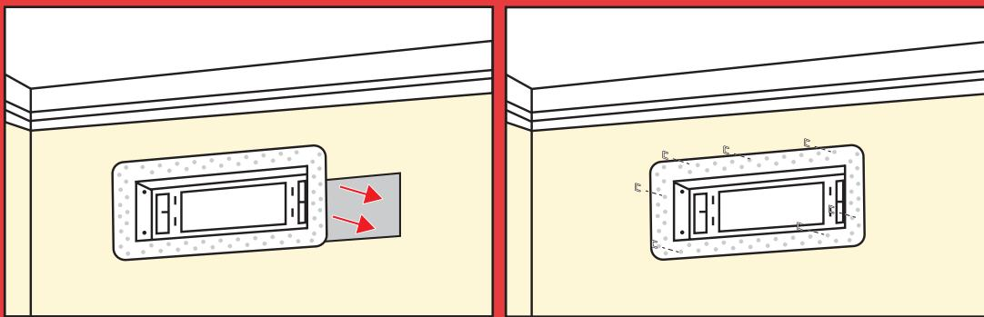
1. Dry fit Drywall Flush Vent into duct opening. Ensure flange is flat to the wall.
