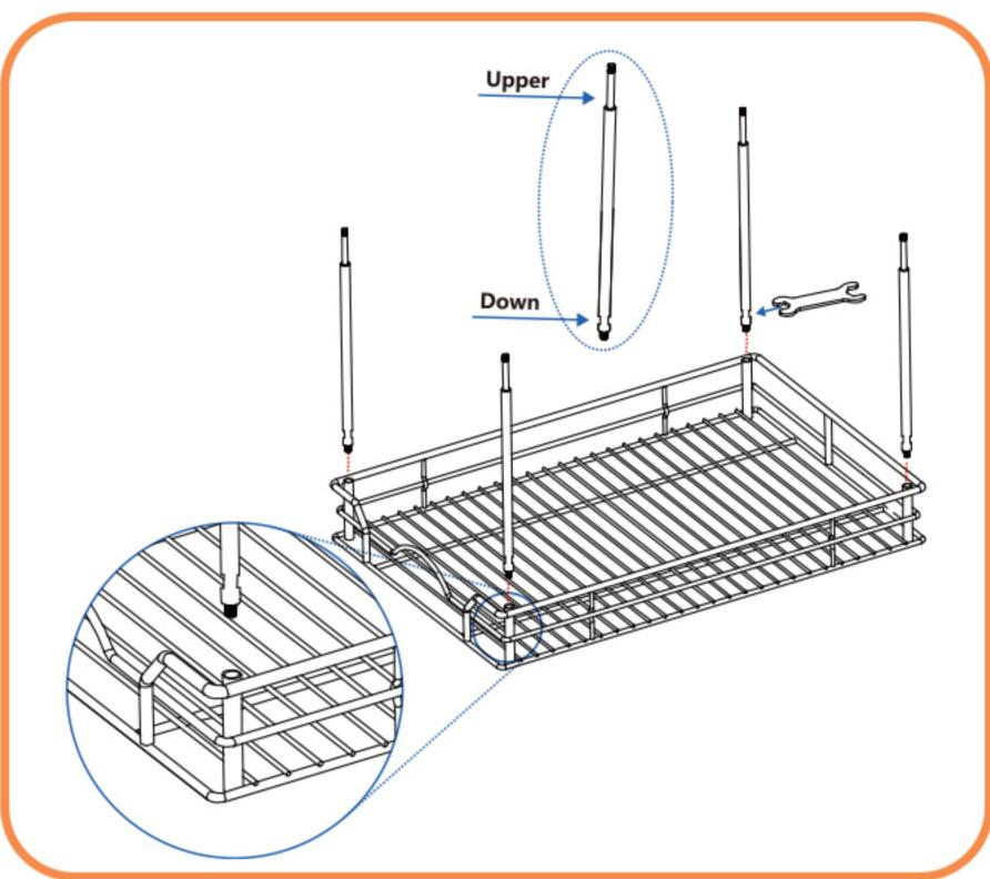
STEP1: Install the screws on the bottom STEP2: Install the connecting rods to of the cabinet using the proofing lower basket card stock
