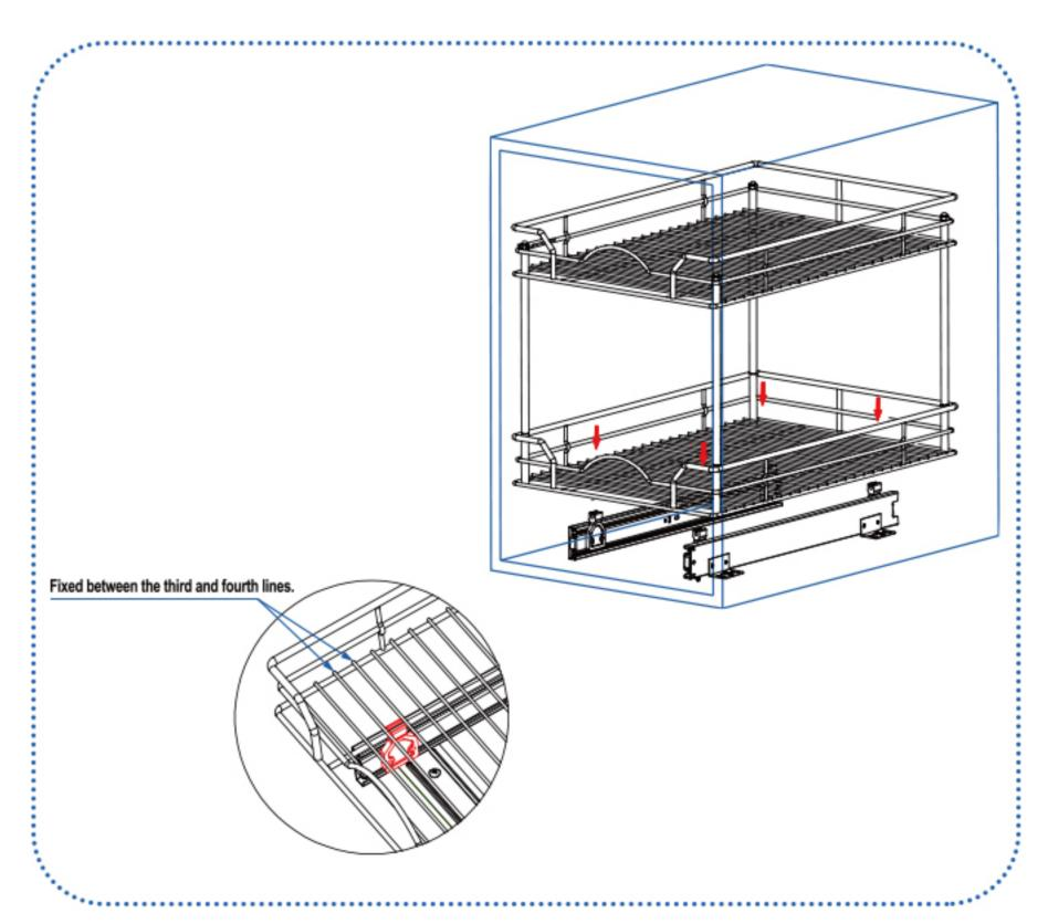
**STEP4:** Install the basket onto the brackets
