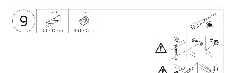
Connect board 6 and 7 to board 8 and 10 using wooden dowel(E), add cam lock(F) into board 8,10 and turn clockwise to tighten as shown.
