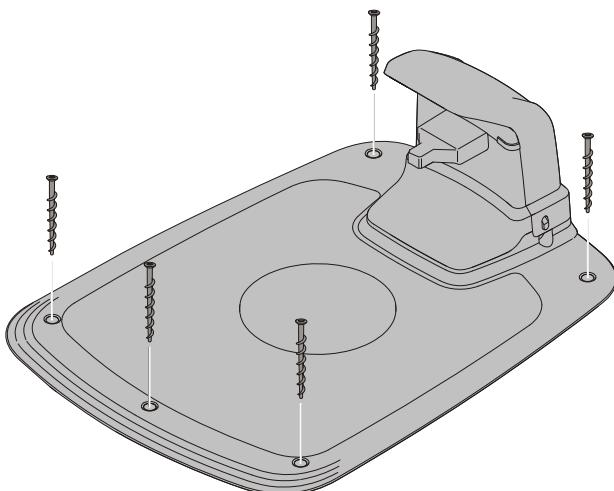
Secure the charging station to the ground using the five supplied fixing screws using a 6 mm hex key.
