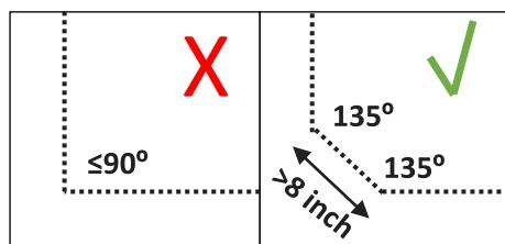
Do not lay the guide wire at sharp angles or the mower will have difficulty following it.
