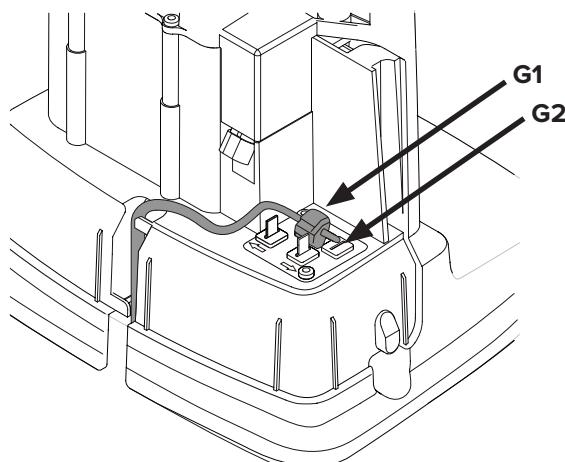
Installation d'un second câble guide (not on all models):
