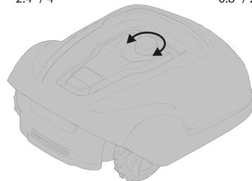
For the first few weeks of mowing, set the cutting height to at least 2.4 inch to avoid cutting the boundary wire and guide wire. Lower the setting one step each week thereafter until the desired cutting height is reached.
