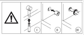
Turn cam locks clockwise to tighten.
