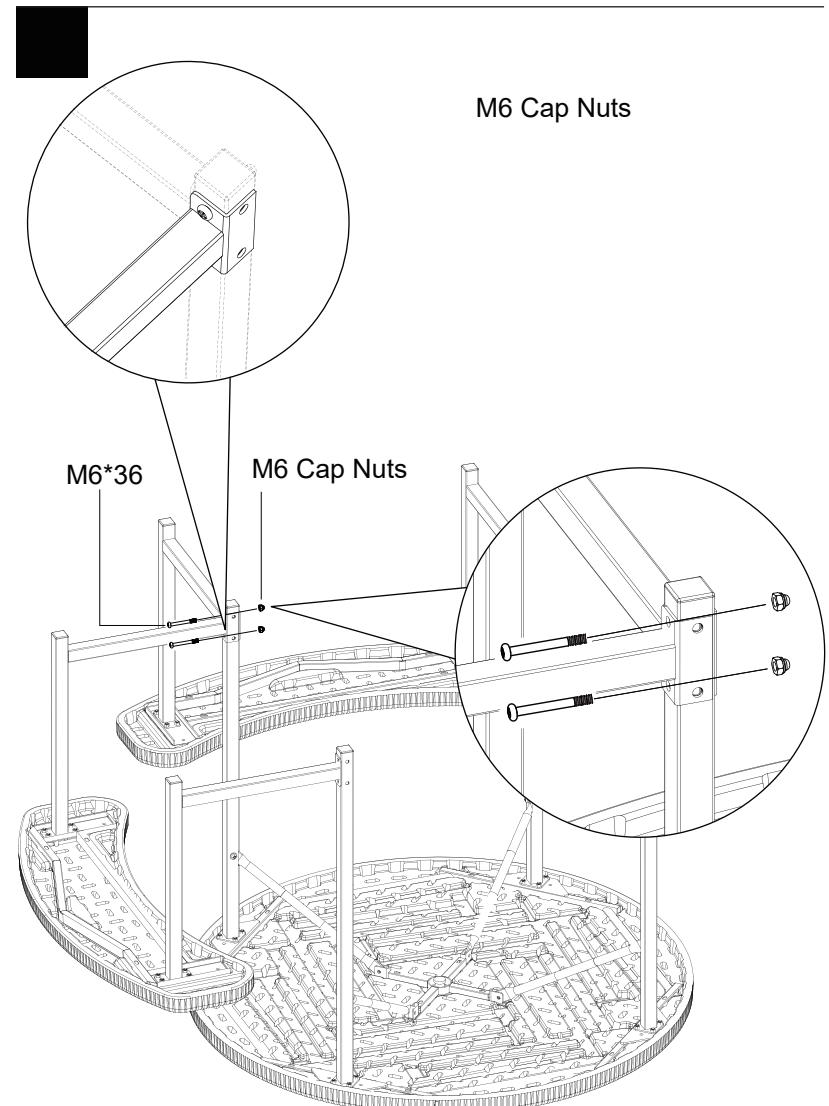
**EN** As shown in the figure, use two M6\*36 bolts and two M6 cap
