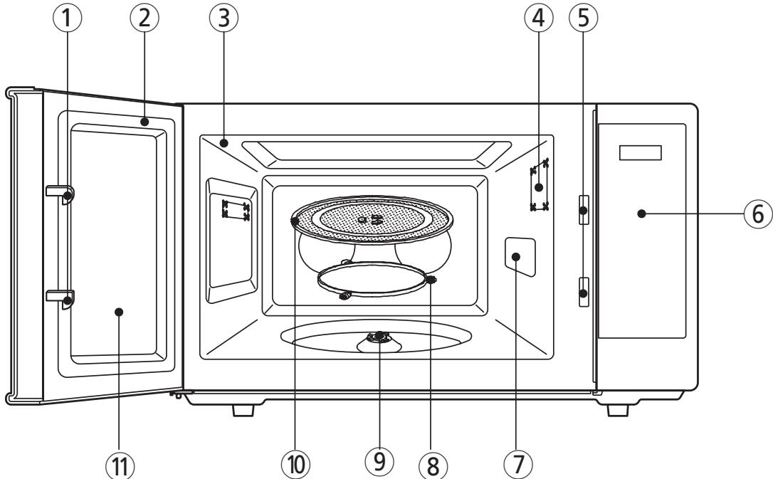
**① Door latch** - If the door is opened while the oven is operating, the magnetron will automatically shut off.
