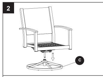
Once all bolts have been installed and hand tightened, go back and tighten firmly with wrench.
