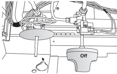
10. Using a butane extension lighter, turn the control knob to LO and light the burner.
